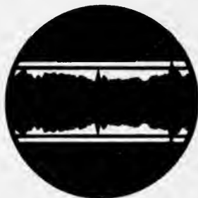
FIG. 5. View through eyepiece showing variable-area track and parallel hairs.
